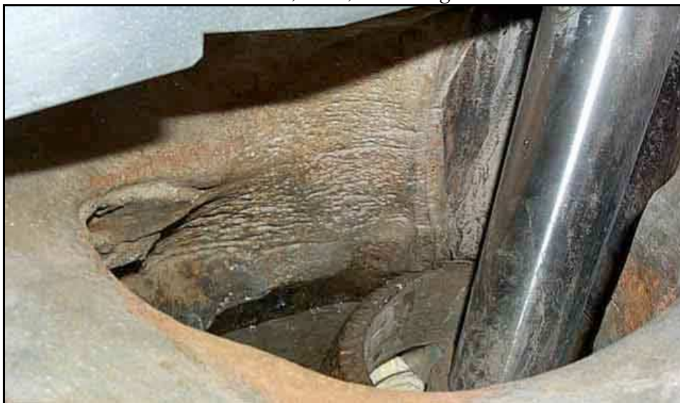
Above and below: Davis-Besse reactor, Ohio, USA: large hole in the reactor vessel head.
